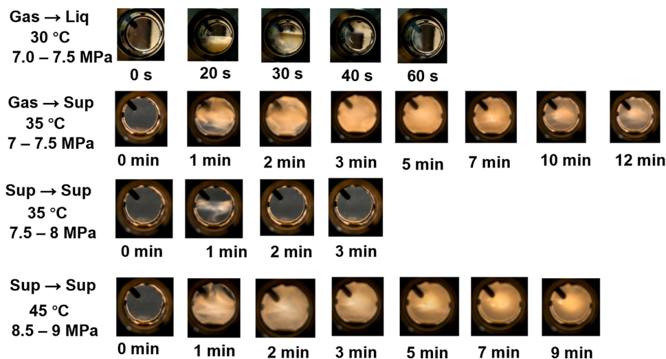
Fig. 7. The phenomena of the flow field with the rise of boost operation time at different conditions, including 7.0 -7.5 MPa (30 °C), 7.0 – 7.5 MPa (35 °C), 7.5 – 8.0 MPa (35 °C) and 8.5 – 9.0 MPa (45 °C).
