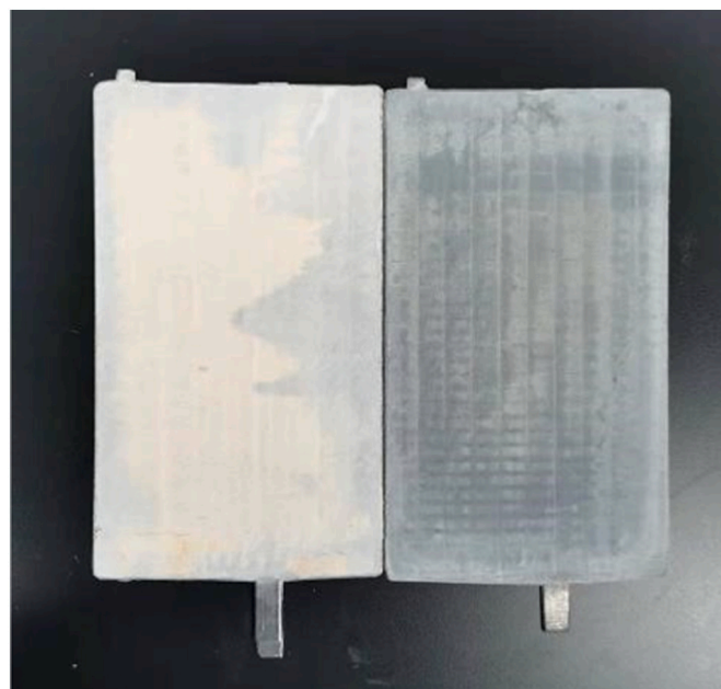
Fig. 2. Positive (left) and negative (right) plate after curing and drying.
